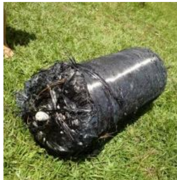
Figure 1. Recovered debris of Falcon 9 second stage, Brazil (December 2014). [4]
