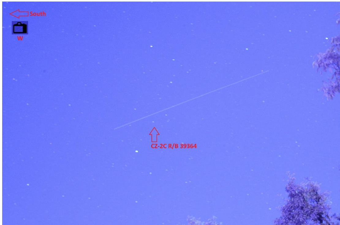
Figure 13. CZ-2C R/B Rocket Body (SATCAT: 39364, COSPAR ID: 2013-059B) orbital debris overpass. Type of orbital debris: derelict launch vehicle stages. Original non-enhanced image. Observation date 14.05.2024. Camera pointed towards west. Overpass direction from south to north. Mean altitude: 314.86 km. [11]
