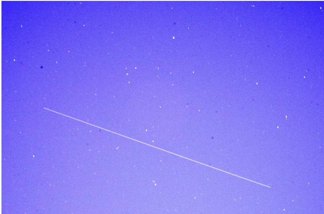
Figure 11. Enhanced image of CZ-2C R/B Rocket Body (SATCAT: 39364, COSPAR ID: 2013-059B) orbital debris overpass. Type of orbital debris: derelict launch vehicle stages. Observation date 12.05.2024. Camera pointed towards east. Overpass direction from south to north.
