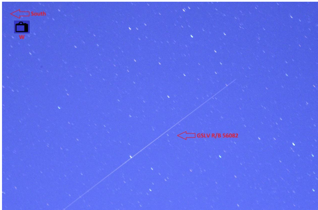
Figure 15. GSLV R/B Rocket Body (SATCAT: 56082, COSPAR ID: 2023-043AN) orbital debris overpass. Type of orbital debris: derelict launch vehicle stages. Original non-enhanced image. Observation date 05.05.2024. Camera pointed towards west. Overpass direction from north to south. Mean altitude: 319.69 km. [11]
